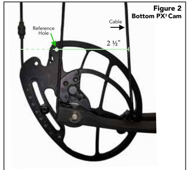
Each XS Plus cam on your Denali bow has a tuning reference hole. The cable on the top cam should be within 1" of the reference hole and on the bottom cam the cable should be within 1" of the reference hole. There is a tolerance of plus or minus 3 twists in each cable and string to optimize tuning. See Figure 3 & 4.
