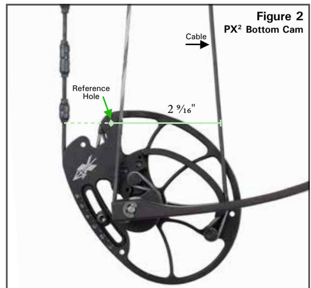
Each XS cam on your Perfexion bow has a tuning reference hole. The cable on the top cam should be within  $1 \frac{3}{16}$ " of the reference hole and on the bottom cam the cable should be within  $\frac{13}{16}$ " of the reference hole. There is a tolerance of plus or minus 3 twists in each cable and string to optimize tuning. See Figure 3 & 4.
